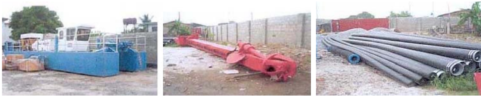
Figure 4b: A 12" x 10" elicott truckable cutterhead suction dredger powered by a 370 hp caterpillar diesel engine, with a 10m ladder and maximum digging depth of 6.1m. Included are 500 metres of 12 inch hdpe pipe with 300 metres of 8 inch hdpe floats.
