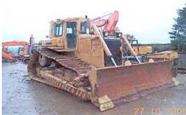
Figure 4c: Caterpillar d6 v-track bulldozer.
