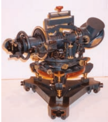
8 inch reflecting theodolite circa 1930. One only of its type designed for use on the Arc of the 30 th Meridian to specifications mostly from Brigadier Martin Hotine. In store at the Science Museum, London.
