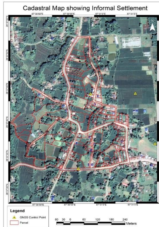
Figure 4: Cadastral map prepared using GNSS control points used for Informal settlement mapping.
