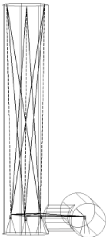
Fig. 5. Connecting measurements from surface to tunnel level
