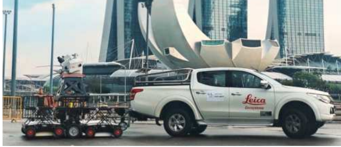
Rapid Ground Penetration Radar for Underground Utility Mapping
