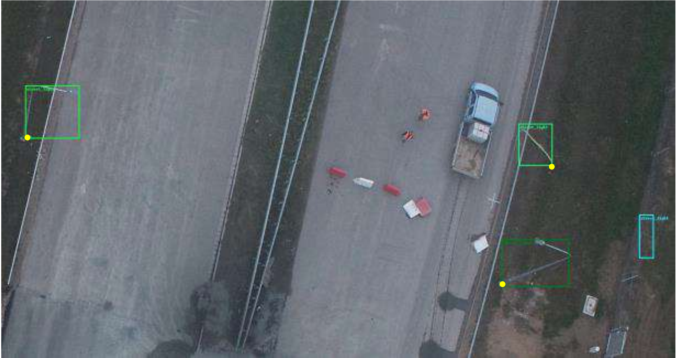
Bounding boxes with approximated location (the closest point to the 2D location of image centre of projection – bottom of the lamp)
