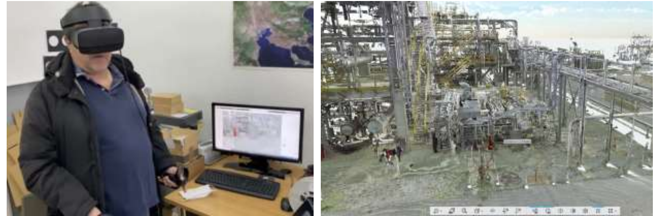
Point Cloud visualization using VR headset and FARO SCENE LT software
