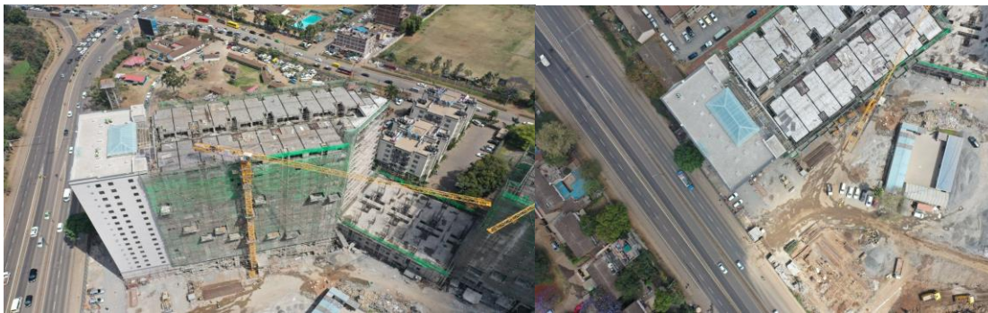
figure: left) image captured drone with camera at a cute angle, right) camera at nadir (90degree) angle
