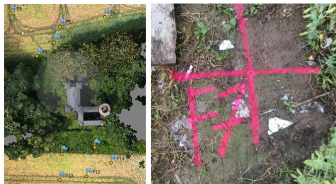
Figure 2. Ground control points network
