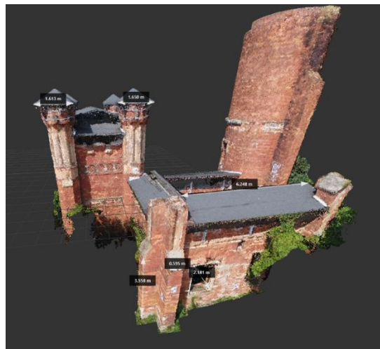
Figure 10. Measurement of the characteristic linear elements of the object on the example of the TLS cloud
