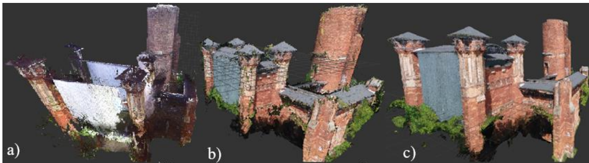
Figure 6. General view of point clouds obtained using: a) TLS b) image data obtained from UAV developed in PIX4D, c) image data obtained from UAV developed in Agisoft.
