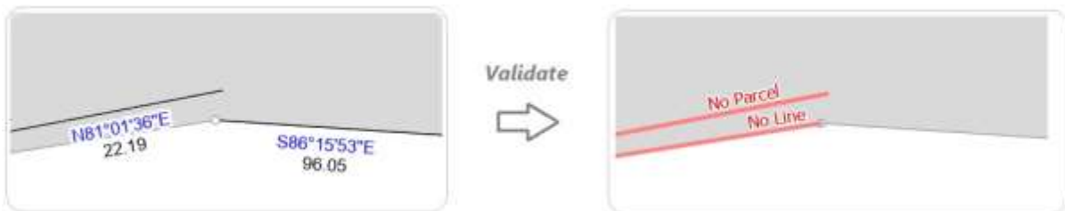
Figure 7. for a parcel type, polygon edges with no line, and lines not on a polygon edge produce line error features
