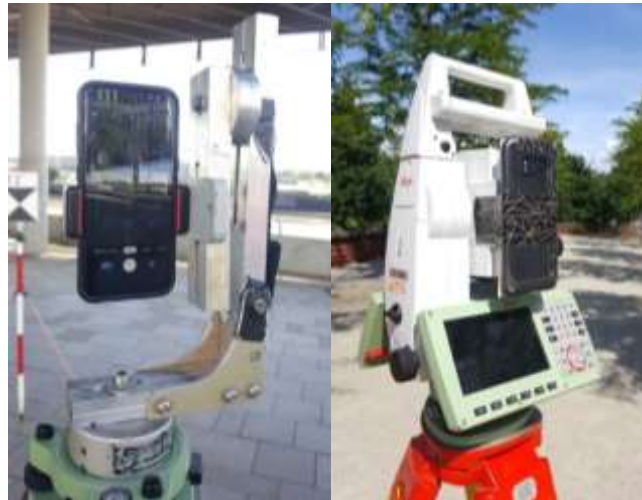
Figure 7: Different Smartphone placements. Left: using the tripod and the holder. Right: Smartphone attached to the TS16
