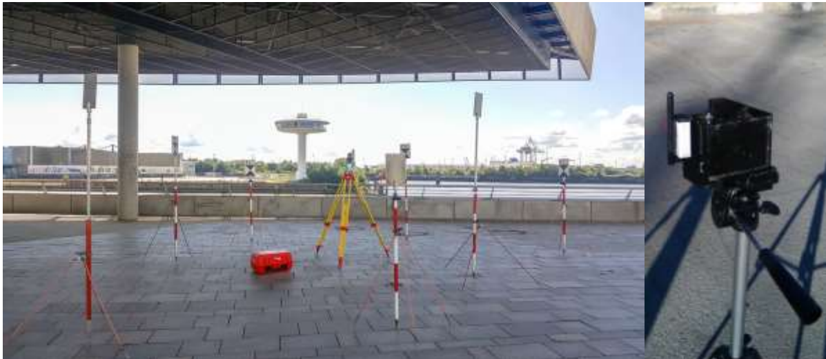
Figure 6: The Measuring field environment. Left: Orientation tracking evaluation. Right: Laser ranging evaluation.
