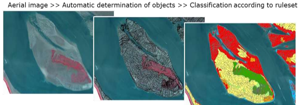
Figure 4: The automated process of making a geomorphological map
