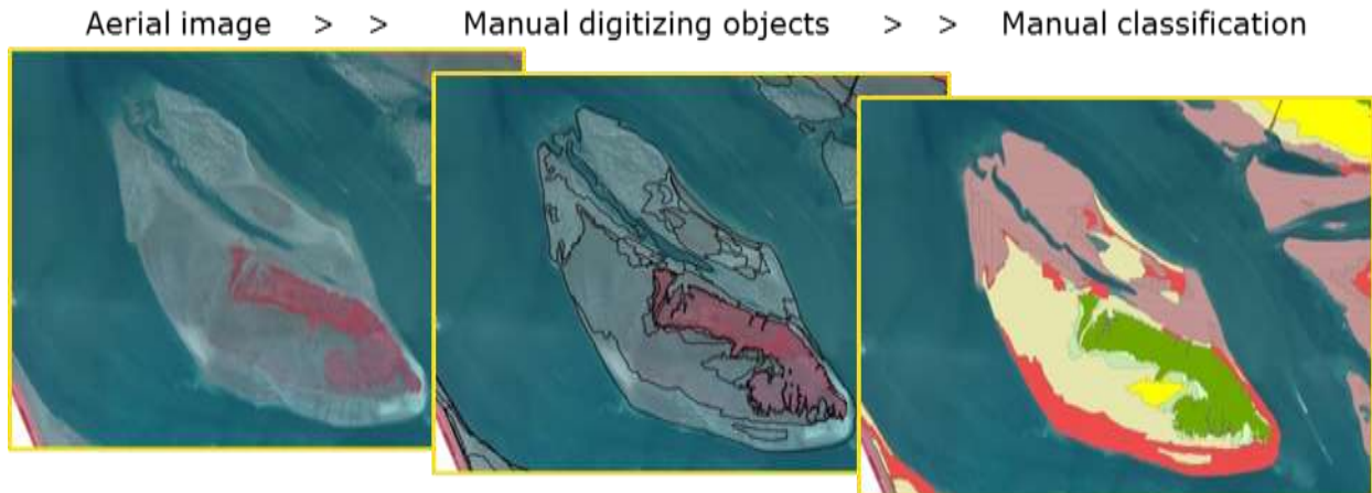
Figure 1: The manual process of making a geomorphological map
