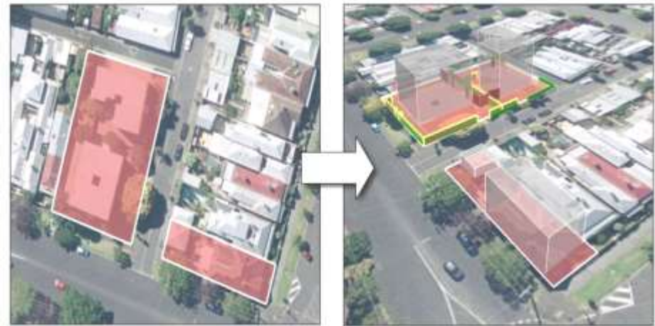
Figure 4. 2D approaches do not enable the complete legal situation on land to be easily understood, for this, need 3D/4D cadastre.
