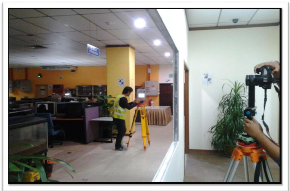
Figure 9: Scanner and clear line of sight to capture all target
