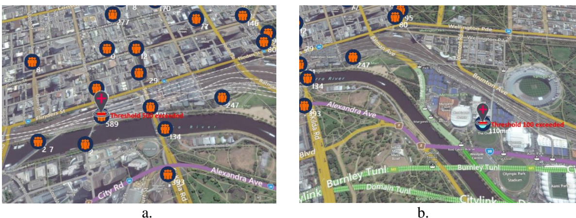
Figure 9: Deployment results: alerts detected by the event identification service for user-set notification rules. a. Shows the alert for pedestrian counting observations where the result of people count observed property exceeded the 500 counts. b. Shows the alert for rainfall observations where the result of rainfall observed property exceeded the 100mm.
