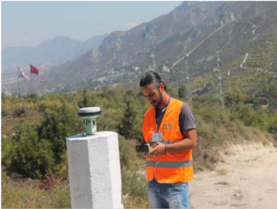
Figure 5.1: GNSS survey on a pillar in TRNC
