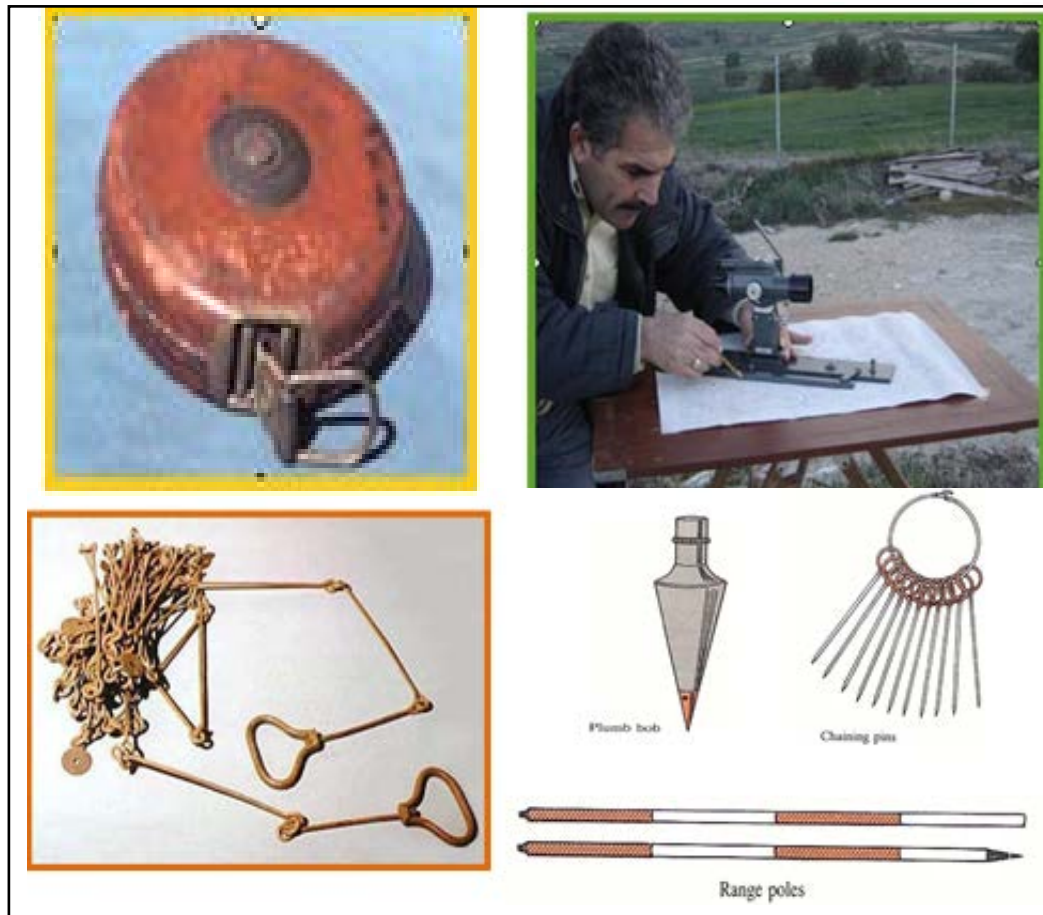
Figure 2.1: Some of the basic tools and Plain table used in the first cadaster (Dr. Elia, E)
