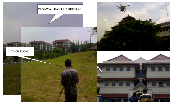
Figure 5. Measurement of vehicle position using Total Station
