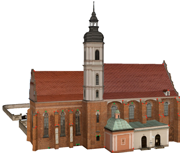
Fig. 3. An example of the location of control points: vector (red) and texture (green) components of the model
