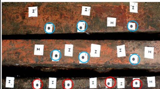
Tie-points: fixed part (in red), mobile part (in blue)
