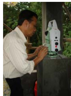
Fig. 4. (a) Design and (b) the first tower for RTS and GNSS CORS at SRM1 station, (c) Setting up of Robotic Total Station
