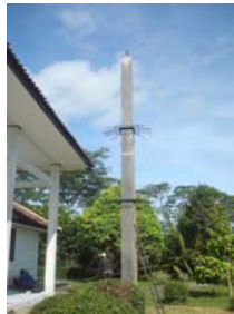
Fig.7. An antenna of the second GNSS CORS and a single of Prism as back sight (a) and (b); (c) box for GNSS CORS receiver at SRM2 station.
