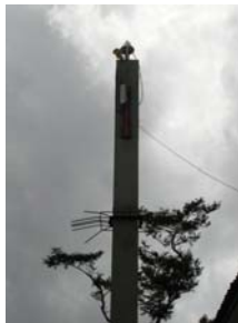
Fig.7. An antenna of the second GNSS CORS and a single of Prism as back sight (a) and (b); (c) box for GNSS CORS receiver at SRM2 station.
