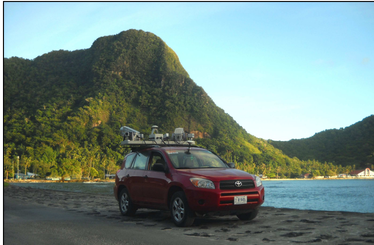
Figure 2: Lynx Mobile Mapper mounted on survey vehicle in American Samoa
