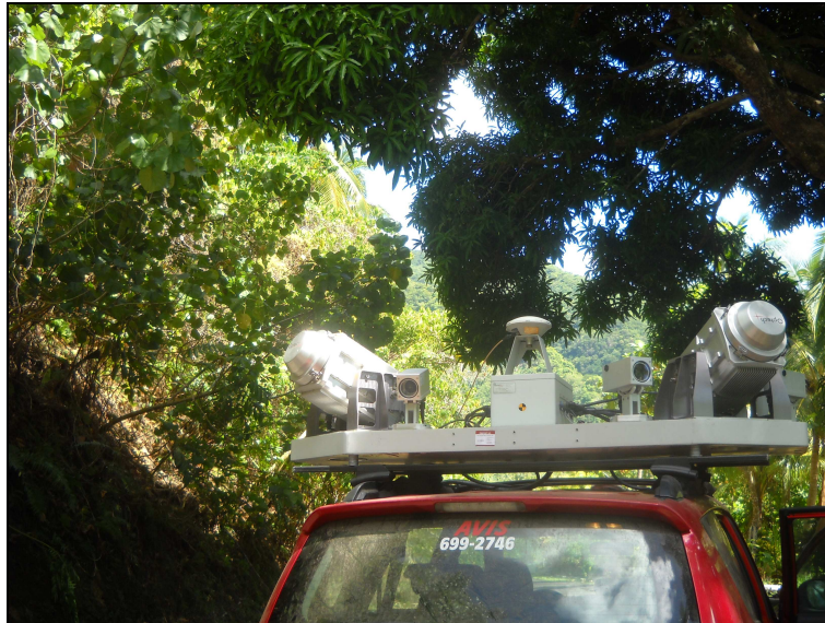
Figure 5: Optech Lynx Mobile Mapper mounted on survey vehicle surrounded by dense vegetation
