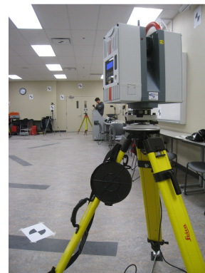
Figure 2: 14 x 11 x 3m Large calibration room
