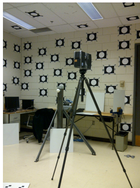
Figure 1: Small 5 x 5 x 3m calibration room
