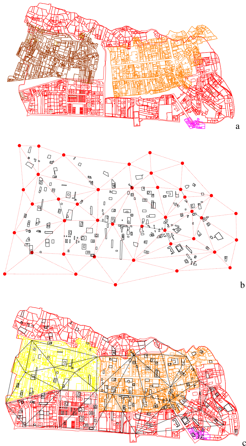
Figure 6 – Map sheets in their actual misaligned reference frame (a); Pregeo surveys framed into the adjusted fiducial network (red dots and dashed lines) (b); Original map sheets realigned by way of the corresponding Pregeo surveys (in black) (c)
