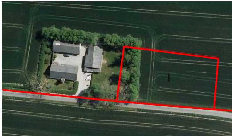
Figure 9: The Danish cadastral map is occasionally very inaccurate due to historical reasons (Kort- og Matrikelstyrelsen 2010)
