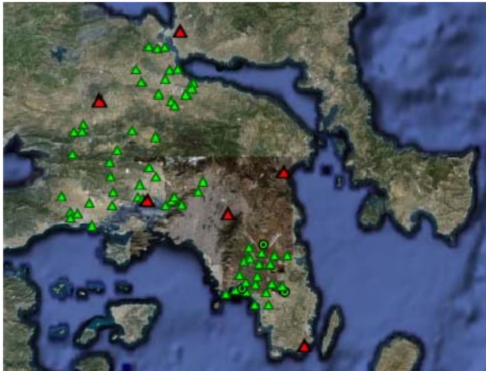
Figure 1: Locations of the GPS/leveling benchmarks (green triangles: trigonometric points, green circles: points of the leveling network, red triangles: HEPOS stations).
