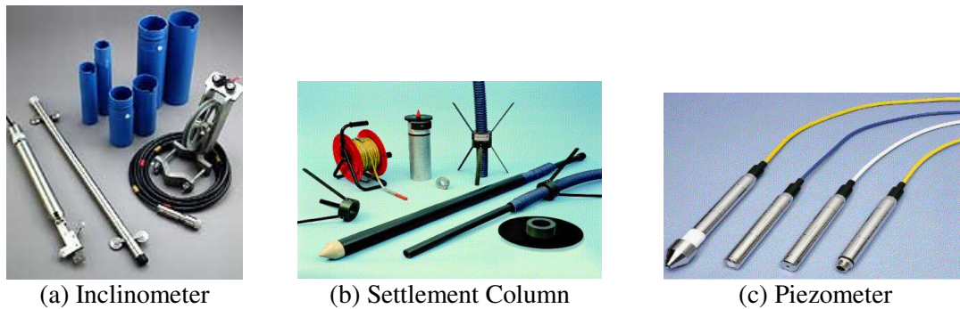
Figure 5a, 5b, 5c. Surveying instruments for non-geodetic method
