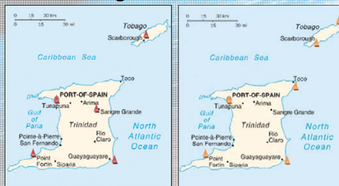
Figure 4 - Distribution of CORS stations (left) and tide gauges (right) in Trinidad & Tobago
