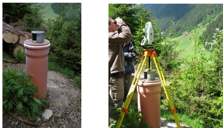
Figure 3: Tacheometer station at the opposite slope
