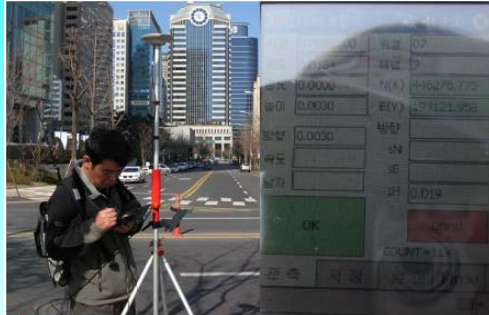
<Figure 3> GPS surveying data received accurately on PDA
