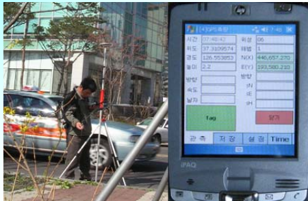
<Figure 2> Correction data not transmitted
