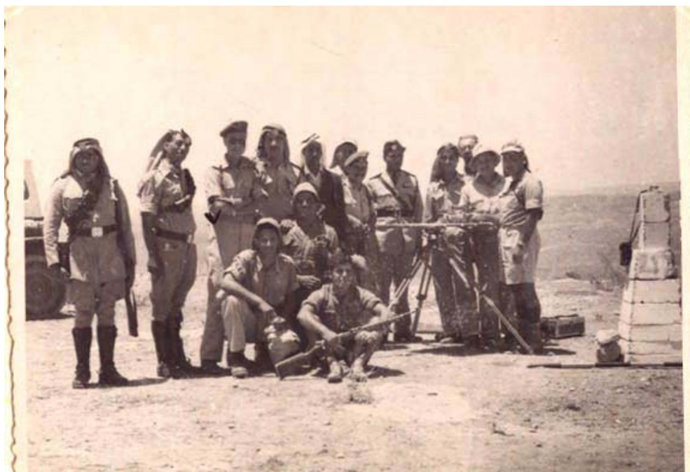
Fig. 21: An example of the bilateral surveying to correct the Armistice Demarcation line. Israelis and Jordanians with a plain table and a border point marker.
