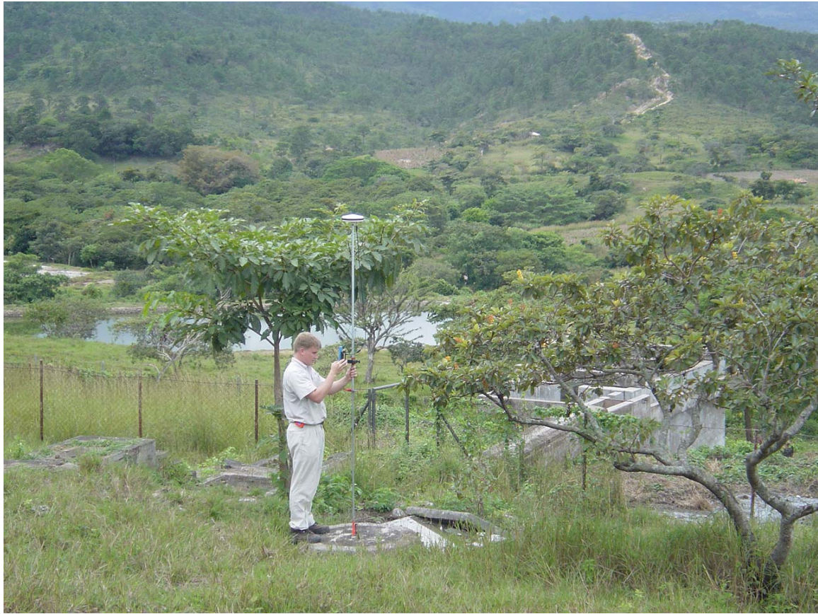
Figure 2: Collecting the coordinates of a storm drain cover in Haiti.
