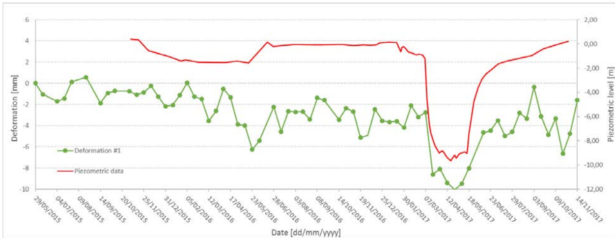
Figure 3. Example of time series that correspond to the maximum deformation area close to the square, shown in Figure 2 (above). From March to June 2017 a terrain subsidence occurs, followed by an uplift to recover to the original height. The pattern of the deformation corresponds well to the pattern of the piezometer level of the same area, shown in red.
