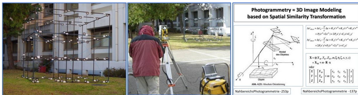
Fig. 13 Calibration Cubic and Total Station measurement : Photogrammetry - 3D Image Modelling
