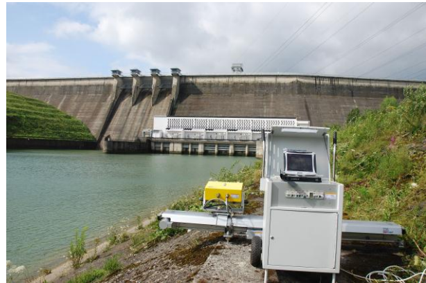
Figure 13. IBIS-L system installed at the second position
