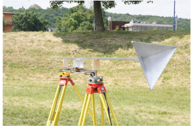
Figure 5. Test platform with microwave reflector attached
