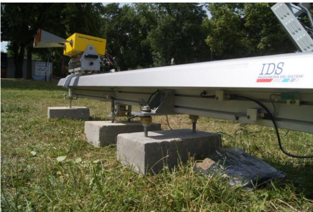
Figure 4. IBIS-L set on the foundation blocks
