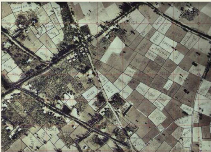
Left: Orthophoto used as a field work map sheet with a georeferenced grid. The map shows the delineated parcel boundaries and parcel identification number. Right: Vectorised field map showing the resulting cadastral map with parcel boundaries and cadastral numbers. Source: Zerfu Hailu, Ethiopia.
