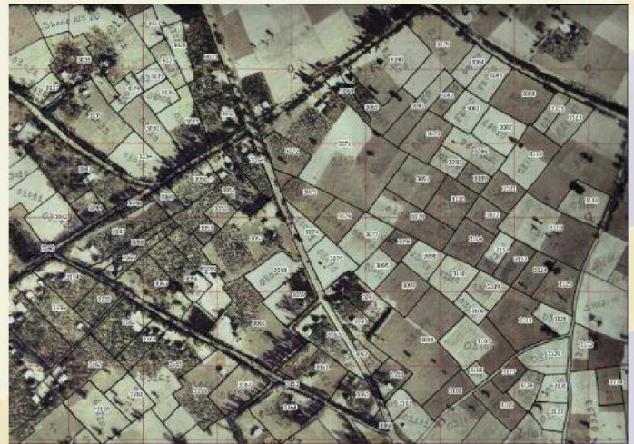
Left: Orthophoto used as a field work map sheet with a georeferenced grid. The map shows the delineated parcel boundaries and parcel identification number. Right: Vectorised field map showing the resulting cadastral map with parcel boundaries and cadastral numbers. Source: Zerfu Hailu, Ethiopia.
