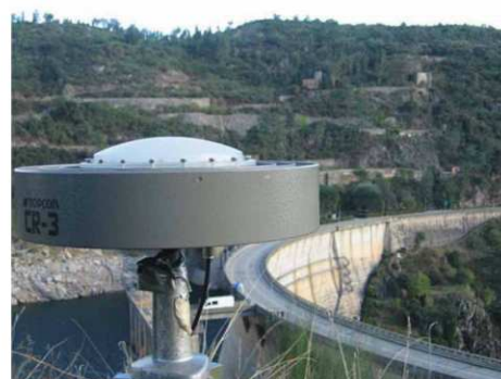
GNSS antenna (reference point) during the continuous monitoring test in 2008.
