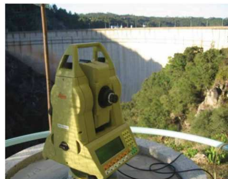
Monitoring the dam in 2008: Tacheometer set on a pillar during the continuous test.
