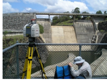
Photo 1: Scanner capturing spillway infrastructure
